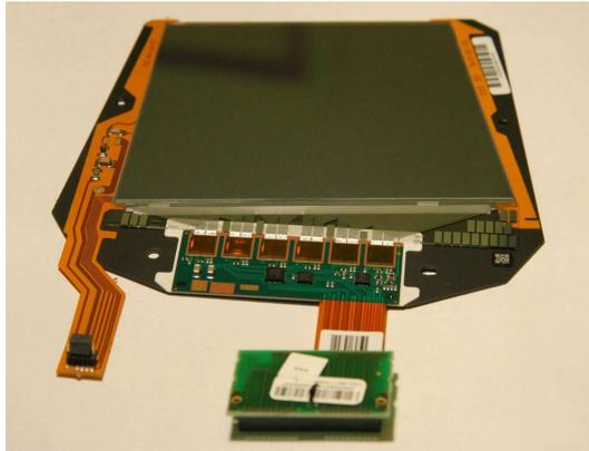
**FIGURE 3.** A module for the TEC subdetector of the CMS silicon tracker.
