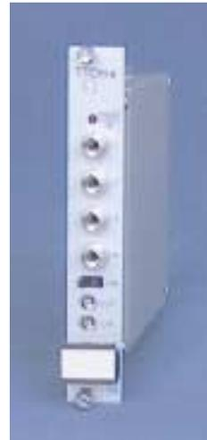
Figure 12: TTCmx laser transmitter
