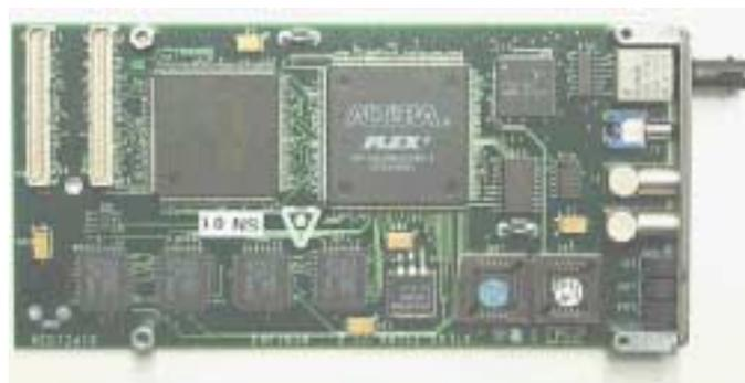
Figure 22: TTCpr PMC receiver module
