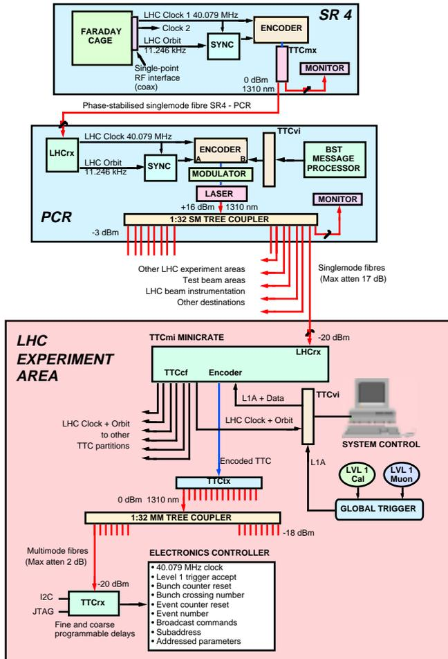
Figure 4: Overall block diagram of TTC distribution
